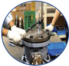
Safety Relief Valve Repair
